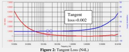
From this figure 3, the tangent loss is 0.002. Hence, the tangent loss is very small.
