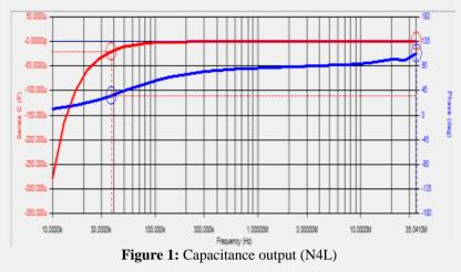
From this figure 2, the negative capacitance proves the substrate material is a meta material. **Tangent loss:**
